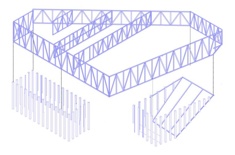
The effect of flying was achieved thanks to the building's design consisting of a combination of iron columns at the bottom and a system of metal trusses at the top, forming a flying bridge at the front and a floating triangle at the rear of the building.
