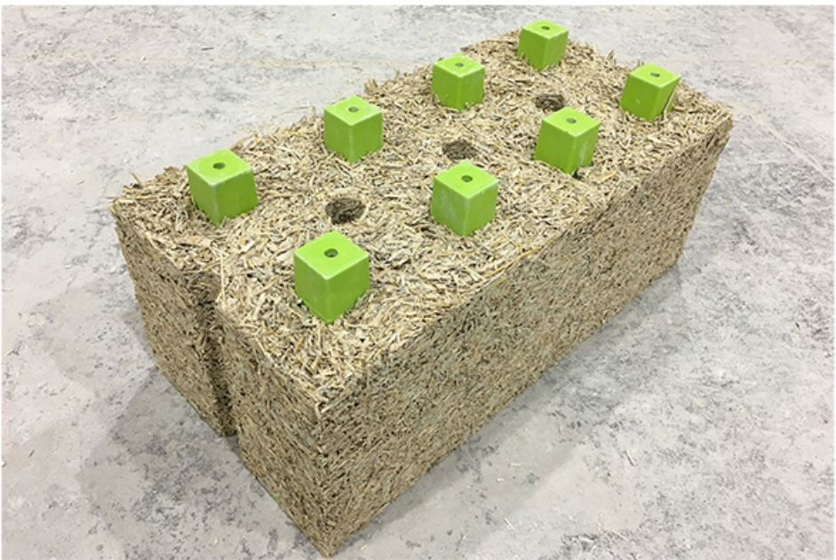
Hempcrete lego style block, idea for revised version of the Walter Segal system.
