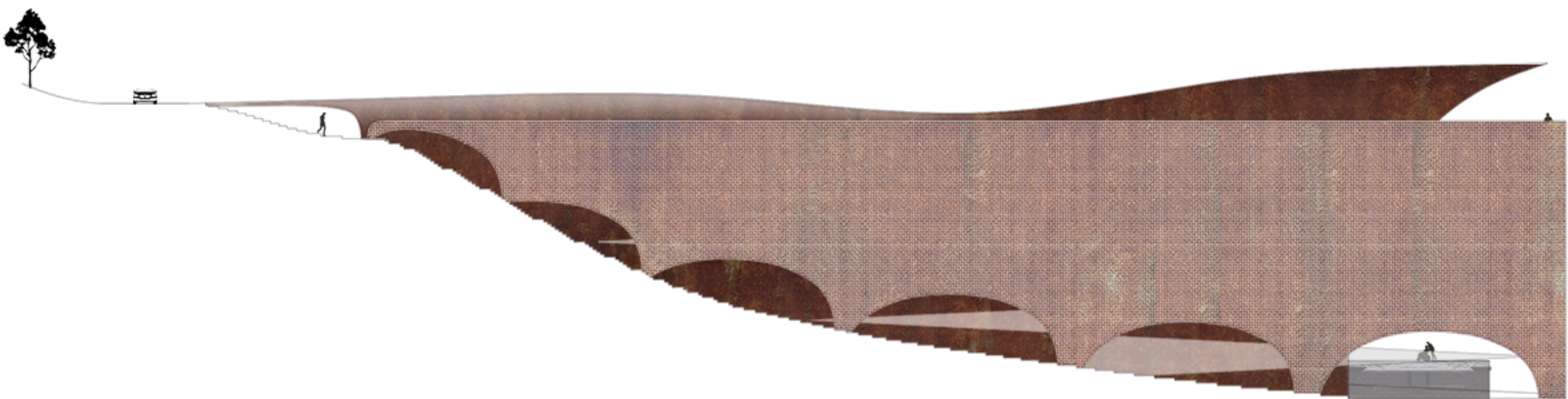
Elevation of the pavilion show context of the road and footpath at the top and ramps running through the outer structure.
